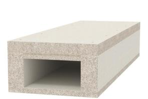
Fire protection duct made from water and frost-proof fibreglass light concrete of building material class A1 according to EN 13501-1 for fireproof laying of cables in rescue and emergency routes, and for the maintenance of electrical functionality of safety-relevant systems. Classification I120 as I duct according to DIN 4102 Part 11 and classification E90 as E duct according to DIN 4102 Part 12.
