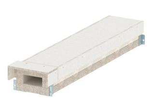
Fire protection duct made from water and frost-proof fibreglass light concrete of building material class A1 according to EN 13501-1 for fireproof laying of cables in rescue and emergency routes, and for the maintenance of electrical functionality of safety-relevant systems. Classification I90 as I duct according to DIN 4102 Part 11 and classification E30 as E duct according to DIN 4102 Part 12.
