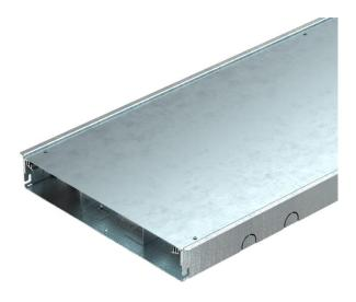
Ready-to-mount trunking unit for cable routing and device installation, consisting of a trunking base with height-adjustable covering contact profile. With mounting protection lid in the as-delivered state. The scope of delivery contains three lid butt seals and a trunking connector.
